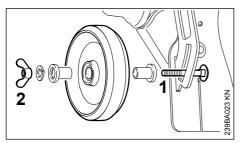
The end of the thread on the screw (1) is peened over to ensure that the wingnut (2) does not work loose and be lost.
