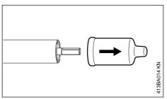
► Pull the protective caps off the ends of the drive tube and keep them in a safe place for later use – see "Storing the Machine".
