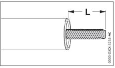
► Push the flexible shaft into the drive tube.
