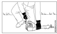
Place the machine on the ground in a secure position
