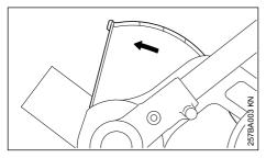
The arrow on the deflector shows the direction of rotation of the blade – see "Using the Unit".
