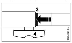
When correctly installed, the red line (3) (arrow point) must be flush with the end of the coupling sleeve.
