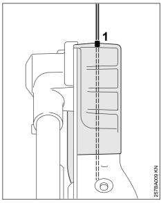
Use the gunning sight (1) to line the blade up with the edge of the bed.
