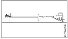
Lay the power edger on its back so that the blade mounting (1) faces up.
